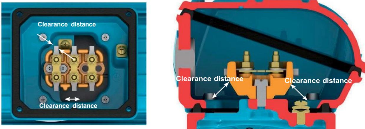
Figure 43 - Minimum clearance distance (mm) x supply voltage
