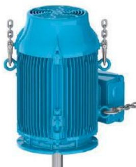
Figure 15 - End result: motor placed in vertical position
