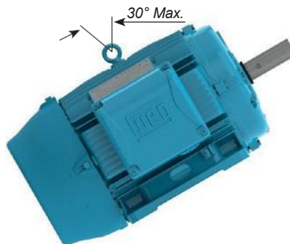
Figure 6 - Maximum allowed angle-of-inclination for motor with one eyebolt
