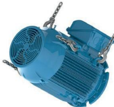
Figure 24 - Motor is being rotated to horizontal position
