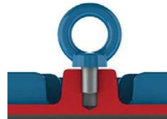
Figure 5 - Incorrect tightening of the eyebolt
