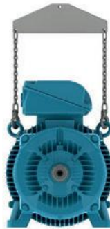
Figure 10 - Use of a spreader beam for lifting
