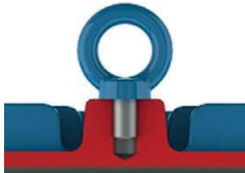
Figure 4 - Correct tightening of the eyebolt
