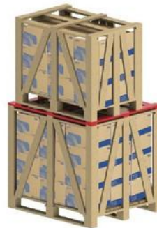
Figure 28 - Use of additional battens for stacking
