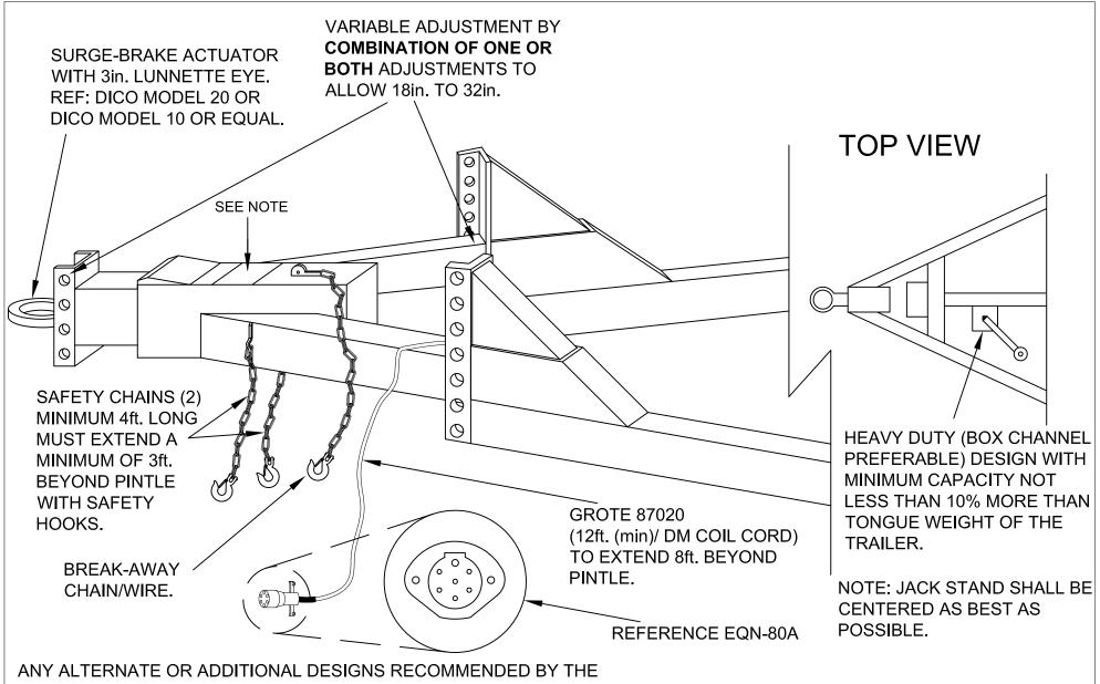
ANY ALTERNATE OR ADDITIONAL DESIGNS RECOMMENDED BY THE MANUFACTURER SHALL BE SUBMITTED, IN WRITING, TO THE FLEET MANAGEMENT DIVISION SPECIFICATION UNIT FOR APPROVAL. IF A PERMANENT HITCH MUST BE UTILIZED IT SHALL BE SET AT 28 INCHES.
