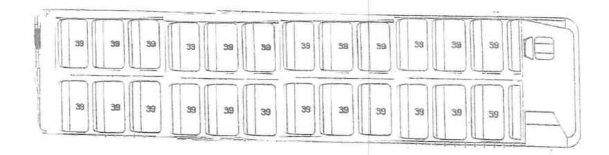
Unit 22-25 - 36 passenger school bus, diesel-fueled, with air-conditioning, Special Ed Options: C, D, H
