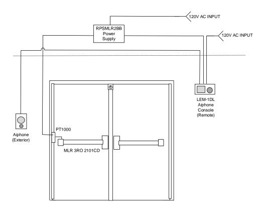
Description of Operation: Access via mechanical key or via Aiphone announcement call. Remote Aiphone console push button initiates latch retraction of exit device. Free egress at all times via exit device touch bar. Exit devices may be dogged for push/pull operation via mechanical cylinder at touch bar.
